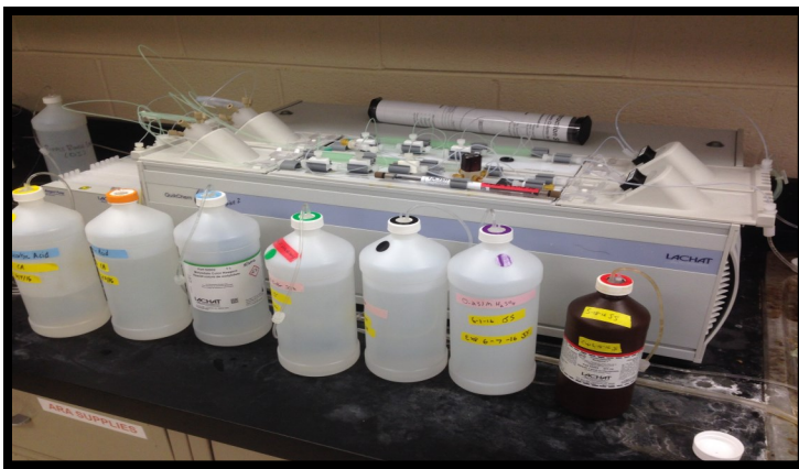
Picture of the Lachat (instrument used for analysis) along with the necessary reagents
